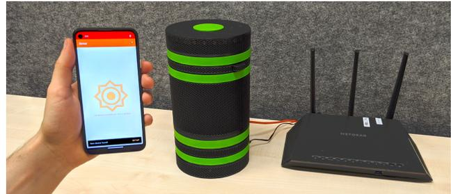
**Figure 1: The user can securely setup a smart speaker. The pairing process involves an acoustic out-of-band channel to protect the integrity of the main channel.**
